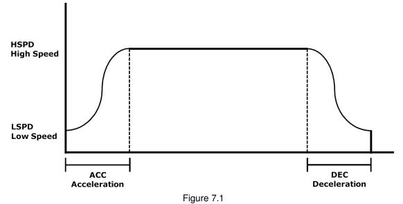
Once a typical move is issued, the motor will immediately start moving at the low speed setting and accelerate to the high speed. Once at high speed, the motor
