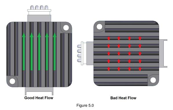
DMX-UMD has a temperature sensor to detect over heating of the driver. Temperature sensing is done only when the driver is enabled. When the temperature goes over the over-temperature alarm value 70 C°, the Alarm Output is turned on. If the temperature goes below the 68 C°, the alarm output is turned off. If the temperature goes over 75 C°, the driver is automatically turned off and remained off until the temperature goes below 68 C°.
