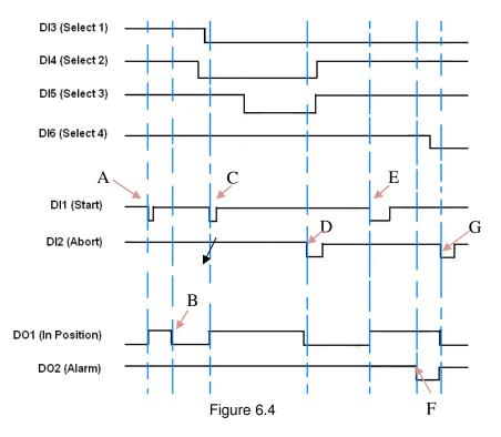
A) On falling edge of **Start**, motion command stored in memory location 0 (0000) is triggered. **In Position** turns off.
